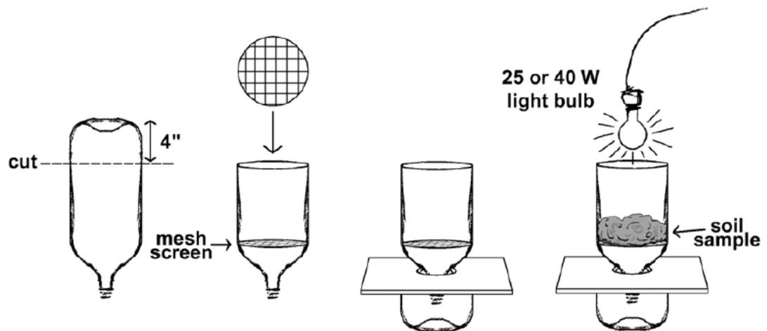
5. Turn on the 25 or 40 watt light bulb and extract for 48 hours (larger samples will require higher wattage and longer extraction times).
